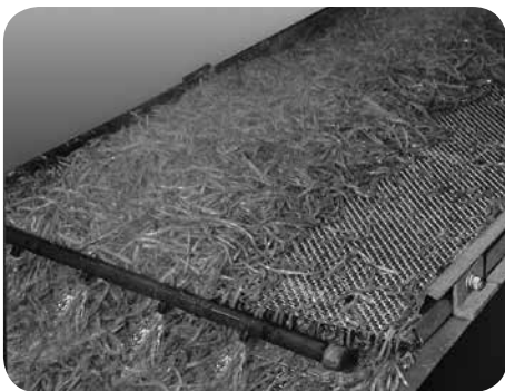
Vibrating screen being used in vegetable processing.
